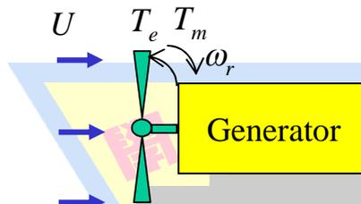
For the direct drive wind turbine system  $\omega_t = \omega_r$  where:
